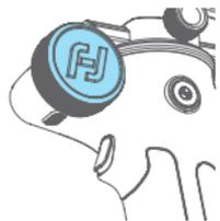
Set current control option as option (1) or (2) or (3) through long press the knob function switching button or swipe up in home page.
