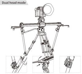
\* After adjusting the use angle, all knobs and joints must be locked
