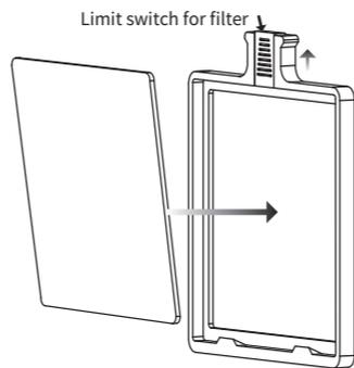
**Filter installation guide:** Move the limit switch at the top of the filter holder upwards until it stops. Insert the filter into the position slot. Ensure that the filter tray is tightly attached, then release the limit switch.
