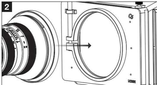
2. Insert the adapter ring into the C5 matte box adapter ring mount.
