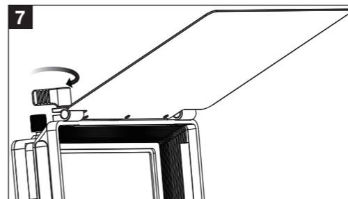
7. The top flag of the C5 matte box can be adjusted accurately at any angle. After adjusting to a suitable angle, tighten the screw of top flag clockwise to lock it securely.
