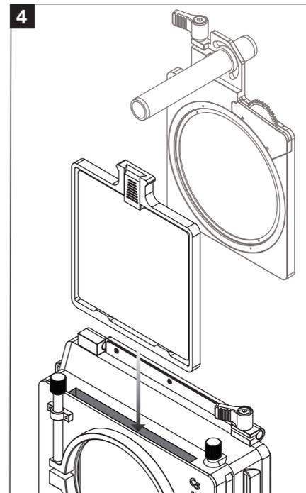
4. Insert the C501-103A or C5 VND into the mounting slot on the top of C5 matte box.
