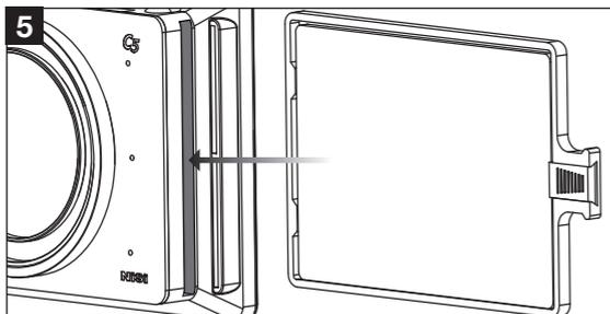
5. Insert C501-102A into the mounting slot on the side of the C5 matte box.
