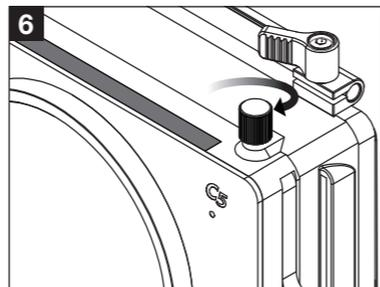
6. Tighten the locking screw for the mounting slot of C501-102A. This locks it securely to the C5 matte box.
