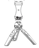
If you are shooting video on your smartphone, mount the phone clip on the tripod, attach the Pocket Wireless device to the cold shoe, plug in the cable and you are ready to shoot.
